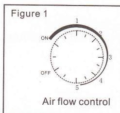
When the ion blower is fixed completely, please check the power cord and turn on the blower. The blower is turned on when you hear a "Pa" sound. At this time, the ion indicator is on. At the beginning, the air speed is maximal. You can adjust the speed according to the practical situation.
