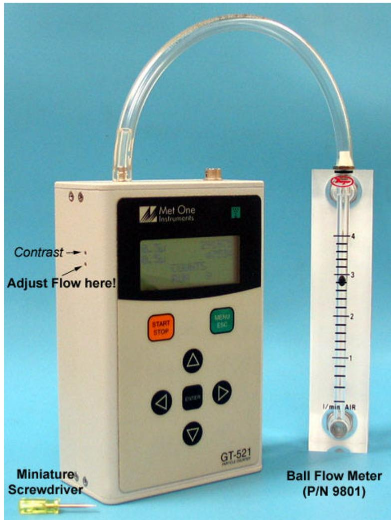
1. To test the flow rate, connect a flow meter to the sample inlet nozzle of the GT-521 using a short piece of flexible 1/8 " ID tubing, Tygon tubing is a good choice.
