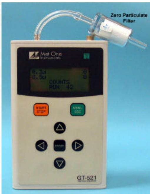
1. Attach a filter with a rating of 0.2 $\mu$ m or better to the GT-521 inlet nozzle. The filter must be large enough that it does not create a restriction and load down the small vacuum pump inside the GT-521. One zero particulate filter (Part number G3111, see section 2.3) is supplied with the GT-521.
