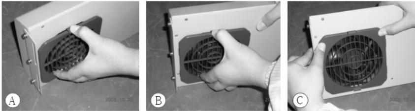
Ⓐ Put the button on the bottom of plastic back cover into the slots of the bottom of metal crust.
