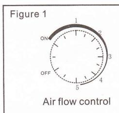
When the ion blower is fixed completely, please check the power cord and turn on blower. The blower is turned on when you hear a "Pa" sound. At this time, the ion indicator is on. At the beginning, the air speed is maximal. You can adjust the speed according to the practical situation.
